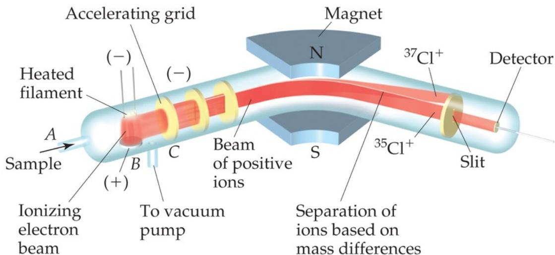
Atomic and molecular masses can be measured with great accuracy using a mass spectrometer.
