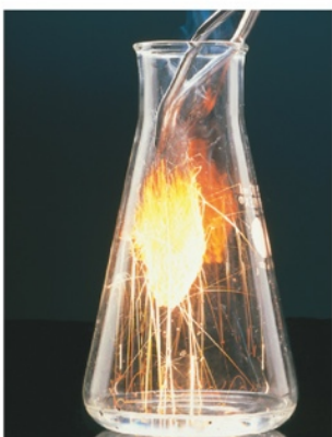
Red-hot steel wool in 100% O_2 burns vigorously, forming Fe_2O_3 quickly
